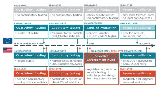
Figure 1: Comparison of the EU and US schemes for vehicle emissions testing
